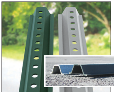
8' Steel Green & Galvanized Posts (1.12#/ft.) 3/8" Holes Drilled Even Inch Available in 6', 7' and 8'
