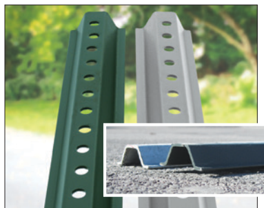
8' Steel Green & Galvanized Posts (1.12#/ft.) 3/8" Holes Drilled Even Inch Available in 6', 7' and 8'
